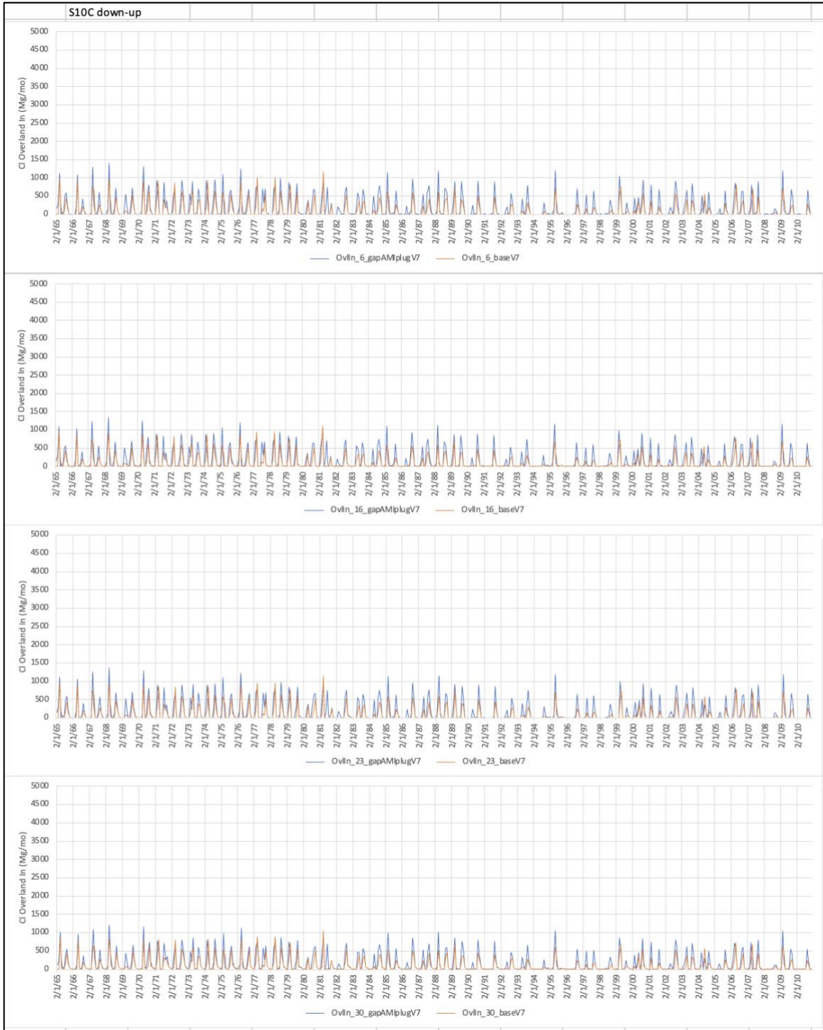
Figure Graph2. Alternative (blue) vs. Base (red) comparative surface water chloride (tracer) inflow budgets in four BIRs along a 1.3 km gradient downstream of the S10 inflow. The Alternative scenario incorporates the Gaps, AMI, and Plug. See above text for details.
