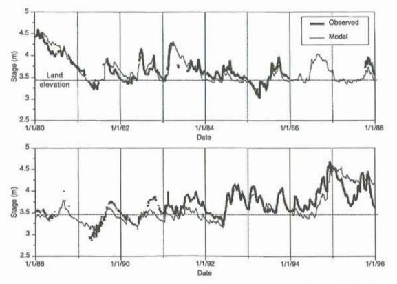
FIGURE 26.8 Simulated and observed water stage at the 2-17 gauge in the central region of WCA-2A (close to site U3 in Plate 26.1). The overall correlation coefficient (R<sup>2</sup>) of the model fit to observed data is 0.70. There are a number of periods (e.g., 1986) for which we could not obtain observed data.
