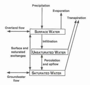
FIGURE 26.6 Water storages and flows for the hydrologic module. The depths associated with water in surface, unsaturated, and saturated storages all vary dynamically.
