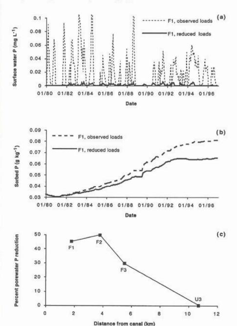
FIGURE 26.15 Simulated surface water and soil nutrient concentrations under the nominal condition of observed P loads and under the reduced-load condition. (a) Surface water P concentration at the F1 (eutrophic) site. (b) Sorbed P concentrations at the F1 site. (c) Reduction, relative to the nominal simulation, in porewater P concentration with distance from the S-10 inflow structures.
